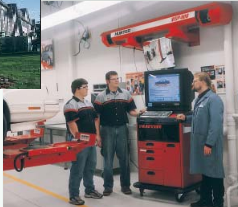
Baker College instructor Scott Spencer and students begin an alignment procedure using the school's new Hunter 611P Plus Aligner and DSP400WMS wall-mount sensors.
