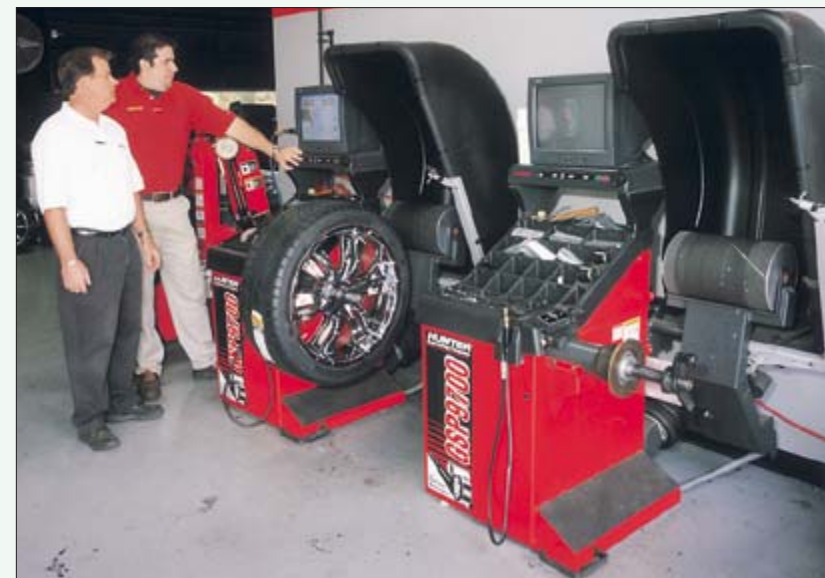
TK Performance technicians use these newest generation GSP9700 Vibration Control Systems to expertly match-mount and balance wheels retailing for thousands of dollars a set.
